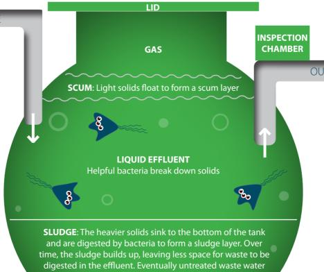
containing heavy solids will flow out of your tank, clogging your soakaway and contaminating the environment.
